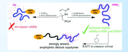
We have recently developed an easy method based on converting a charged monomer (AMPS) to a ionic liquid by neutralization with a tertiary amine<sup>\*</sup>, allowing to introduce a polystyrene block.
